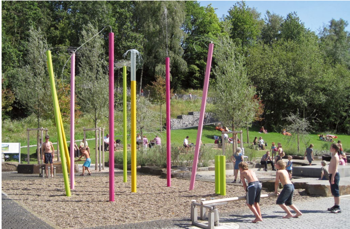
Masts made of stainless steel, powder-coated
